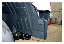
10. Remove steel bumper bar reinforcement.
