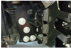
NOTE: Before tightening, adjust bull bar mounts so that the mounting faces for the bar are 815mm apart and centralised to vehicle.
